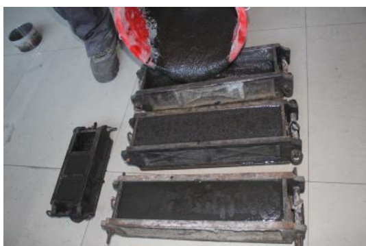
Fig. 2 - Casting drawing of specimens
