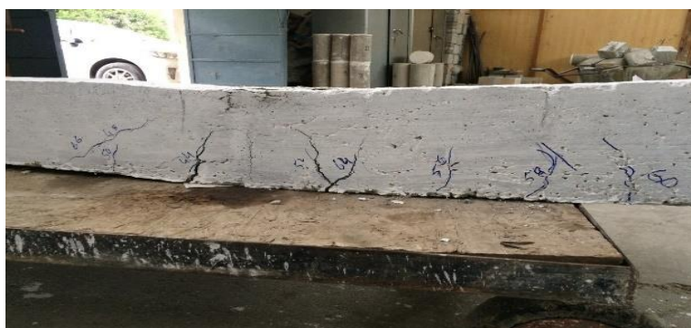
Fig. 8 – Crack pattern in 40% PCA specimen
