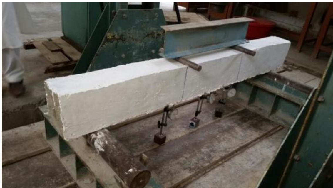
Fig. 4 – Third point loading
