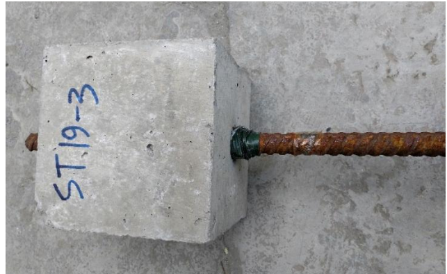
Fig. 18 - Splitting Failure of ST19_3 Specimen
