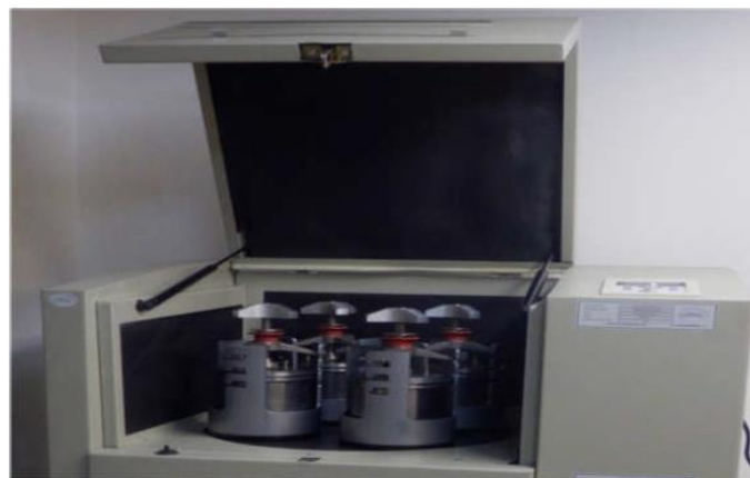
Fig. 2- The ball mill used for the production of micro rubber
