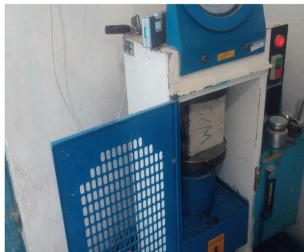
Fig. 5- Testing the specimens' compressive strength
