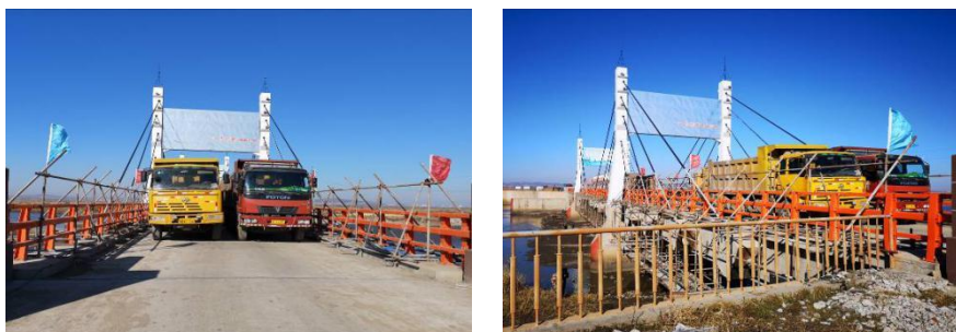
Fig. 7 - On-site loading situation
