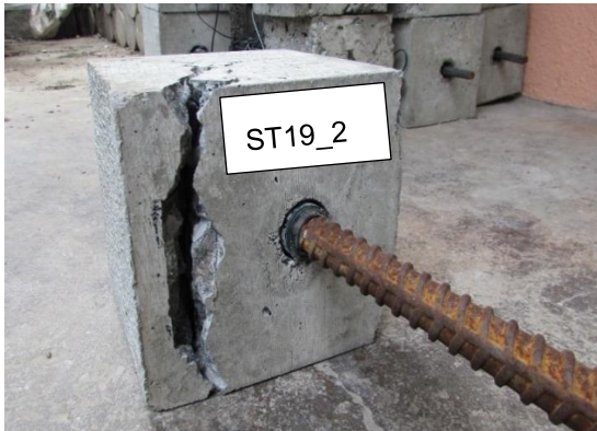
Fig. 17 - Splitting Failure of ST19_2 Specimen
