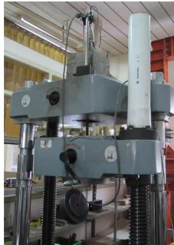
Fig. 6 - Pullout Test Set-Up Using UTM
