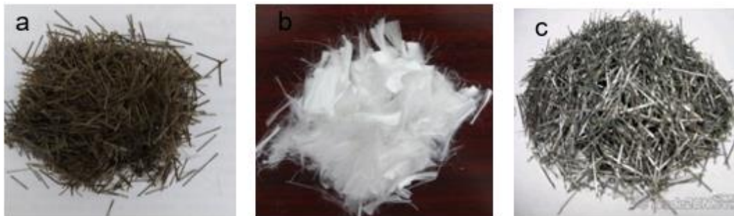
Fig.1- Fiber type: (a) Basalt fiber (b) PP fiber, (c) Steel fiber
