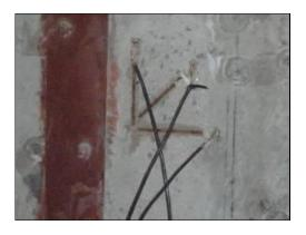
Fig. 24 - Measuring points arrangement of principal stress
