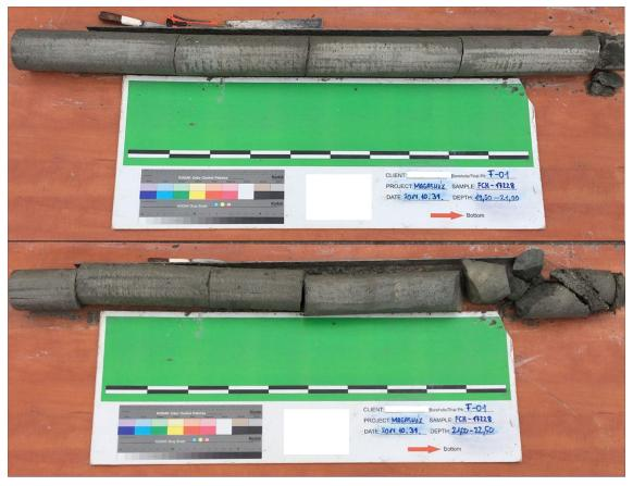
Fig. 2 – Core samples from the top zone of the Kiscell clay layer
