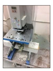
Fig. 6 - Flexural test setup according to ASTM C 348
