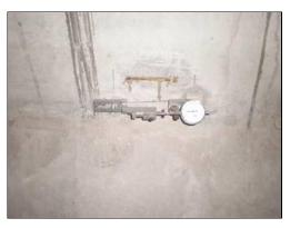
(a) (b) Fig. 23 - Measuring points arrangement of longitudinal stress
