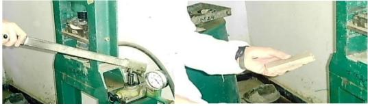
Fig. 6 - Manufacture of pressed bricks
