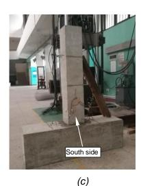
Fig. 4 - Manufacturing process of the precast column: (a). Install of plastic hinge zone; (b). Hoisting of the column; (c). The precast column
