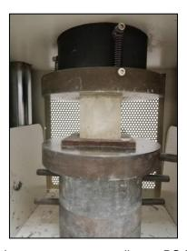
Fig. 5 - Compression test setup according to BS EN 12390-3: 2001
