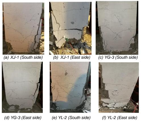
Fig. 7 - Crack patterns and failure mode of the specimens at displacement of  $5\Delta$
