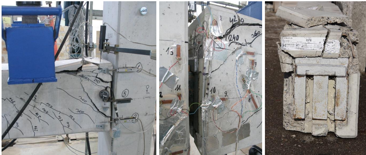
Fig. 7 – Joint failure at reaching the ultimate loading
