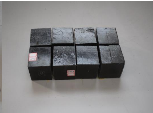
Fig. 2 - Compression strength specimen
