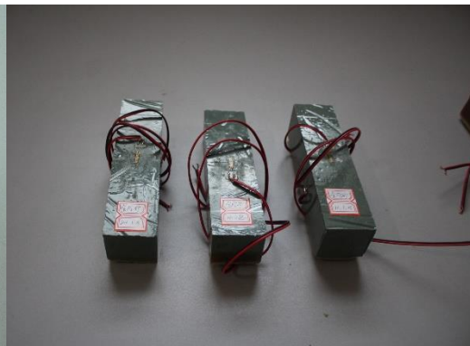
Fig. 4 - Polyurethane emery specimen
