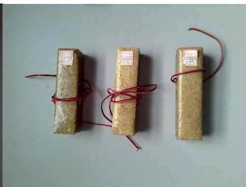
Fig. 6 - Polyurethane lime specimen
