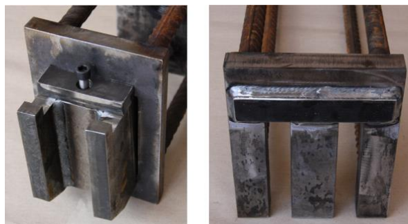
Fig. 3 – Steel fittings embedded in the column including the connecting element (on the left) and the girder (on the right) [3]
