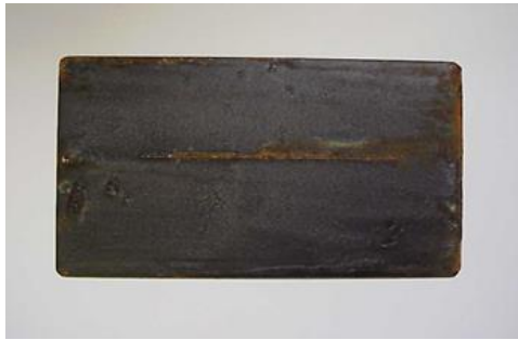
(c) Coal tar epoxy coating with 1 wt.% anion exchange cellulose in SO_4^- form
