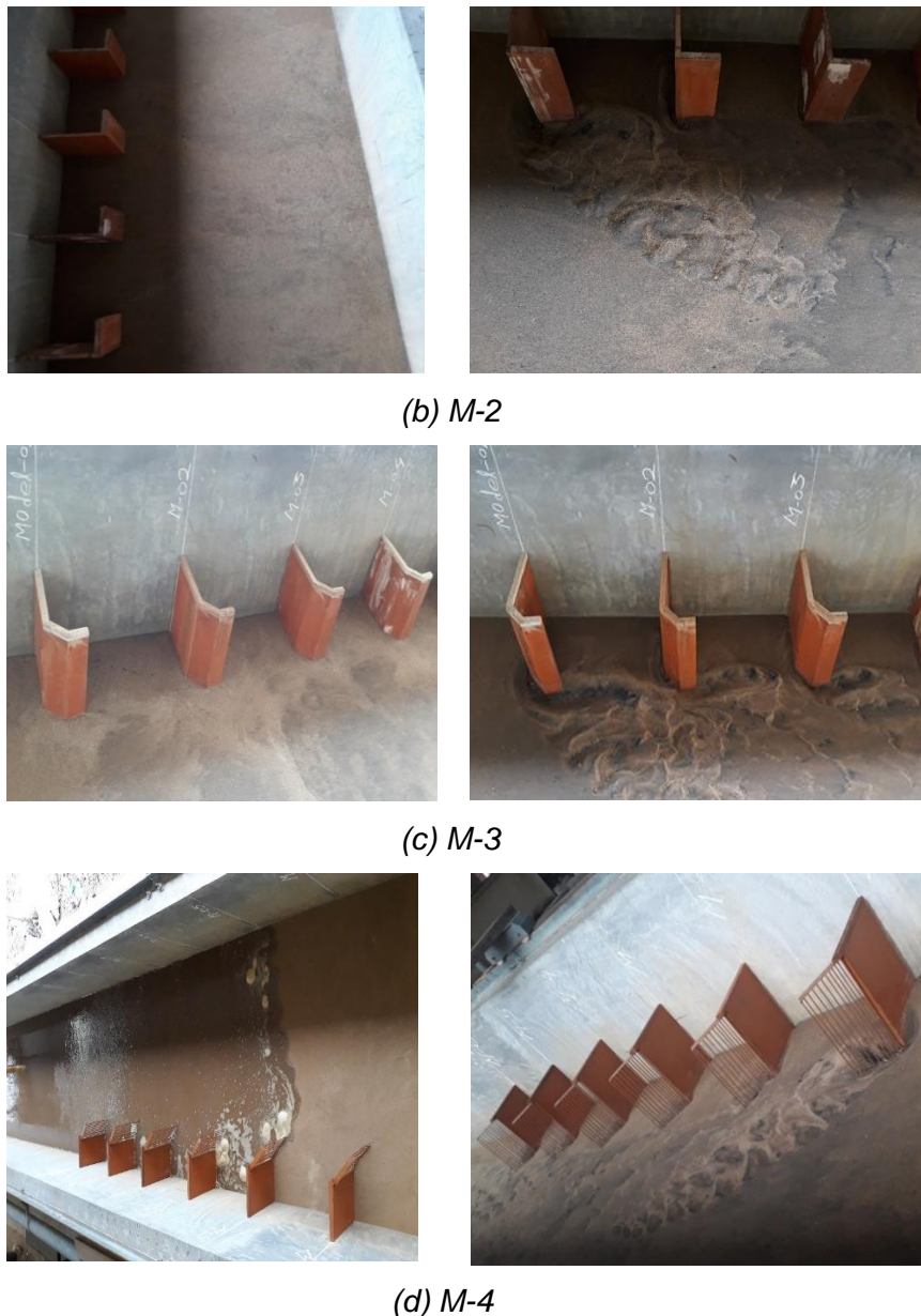
Fig. 3 – Initial bed (left) and final bed (right) with four different groin models: (a) M-1, (b) M-2, (3) M-3, (4) M-4
