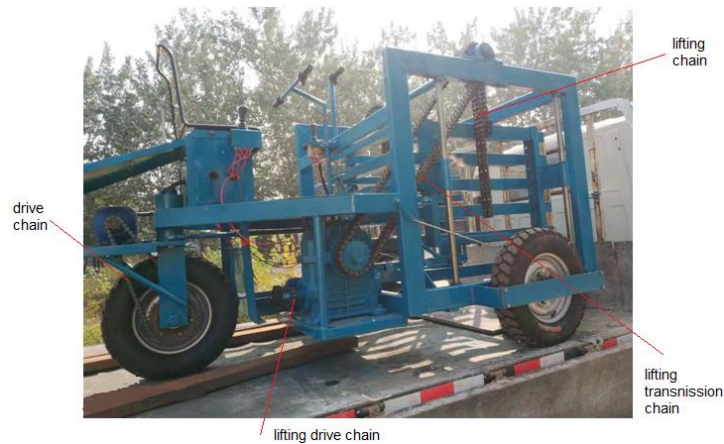
Fig. 10 - All the chains used in the bricks transportation car
