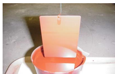
(a) A substrate prepare for coating (b) Withdrawal of substrate from the coating mix
