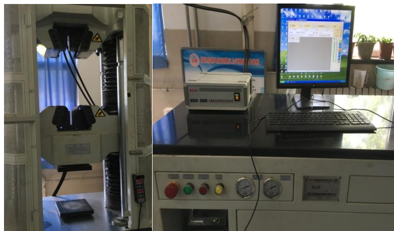
Fig. 5 - WAW-1000 universal testing machine
