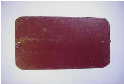
(a) Vinyl coating with 1 wt.% anion exchange cellulose in PO_4^- form
