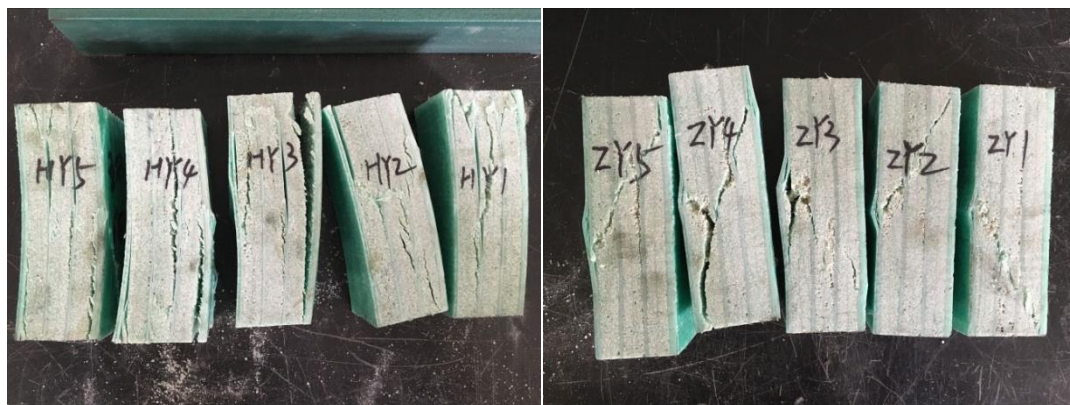
Fig.8 - Failure modes of specimens
