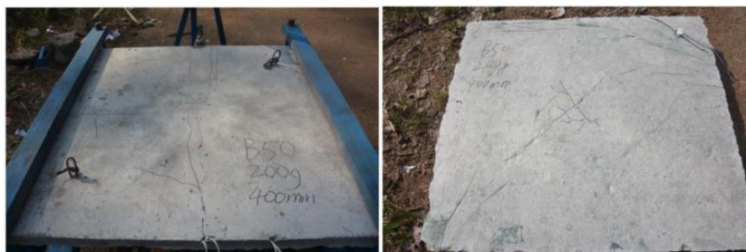
Fig. 6 – Damage patterns of the slabs after physical experiment at top surface (left) and bottom surface (right) [15].
