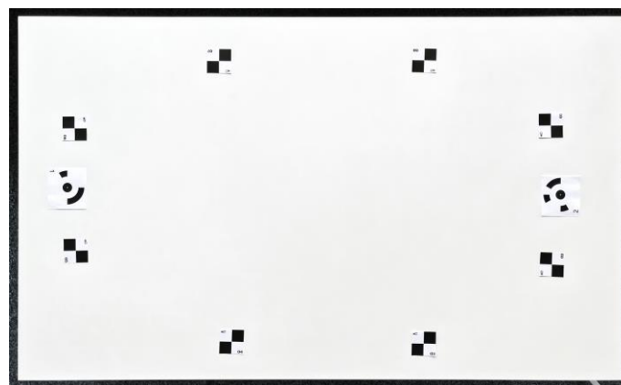
Fig. 4 – Distribution of ground control points on the imaging board (object placed in the center)
