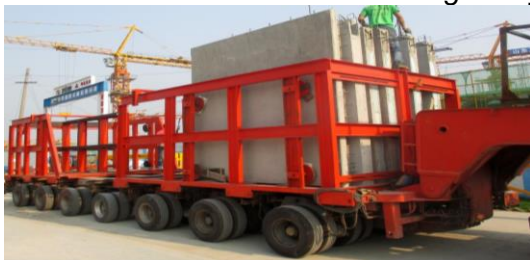
(a) Fixing measures and pads
