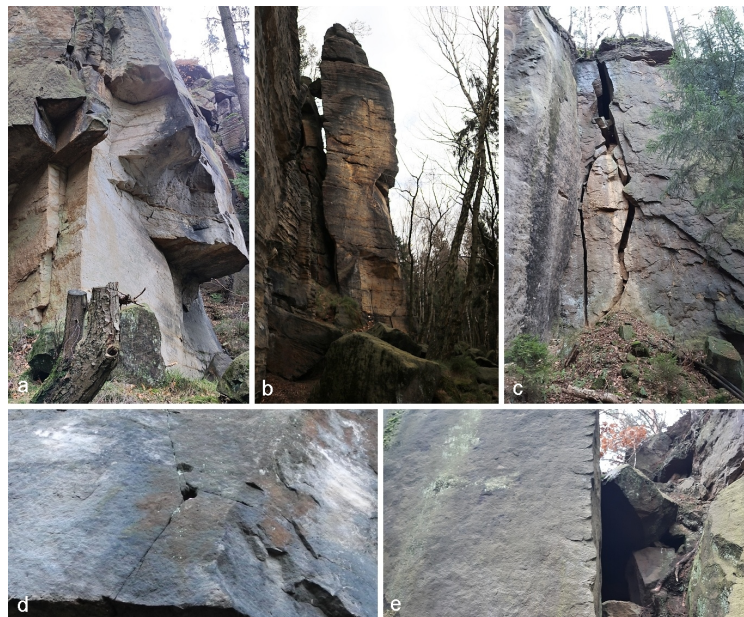
Fig. 1 - Methods of sandstone mining inducing instabilities in rock massifs (examples from the Suchá Kamenice River valley and the adjacent part of the Elbe River canyon: a) a shelf quarry in the valley of the Suchá Kamenice River with well visible traces after quarry-face mining using the technique of undercutting, b) Zlomiskova věž Pillar, produced by extraction of joints and surrounding sandstone blocks, primed for induced fall to the Elbe River canyon by undercutting its base, c) a crevice (dilated tensional joint) formed by unloading of the massif by mining in the Comiteebruch Quarry, d) borings for loading explosive cartridges, e) bags after the insertion of splitters (photo by K. Podroužek)
