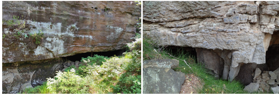
Fig. 2 - Unfinished mining using the undercutting technique in the Elbe River canyon: left) in the area of the Comiteebbruch Quarry, preserved as a deep “overhang” 7×3 m in size; right: unstable rock wall in the whetstone quarry near Podskalí (photo by Z. Vařilová)
