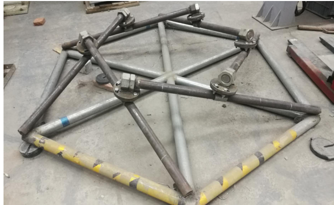
Fig. 5 - Single-layer reciprocal frame
