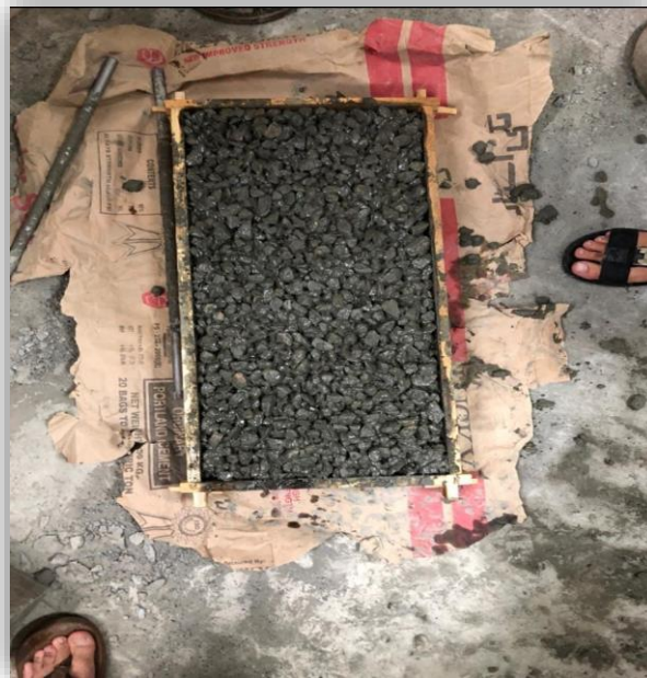
Fig. 3 – Slab placed in its Custom Wooden Mould
