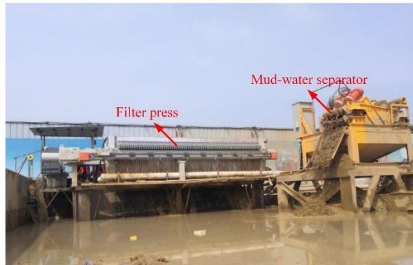
Fig. 5 – Slurry separator and press filter
