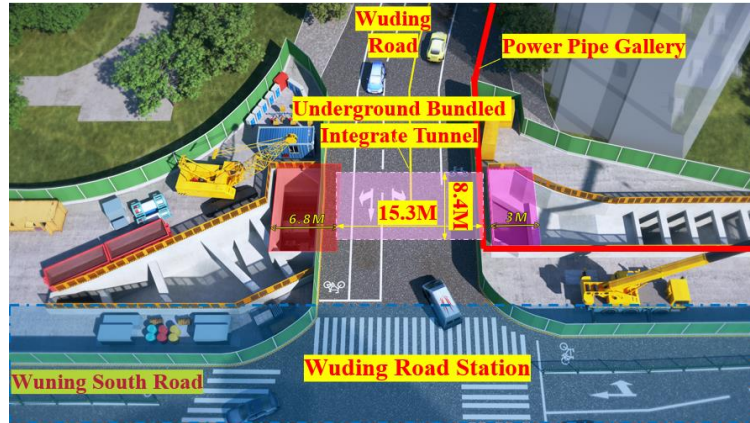
Fig.4-1 Plane graph of underground bundled integrate tunnel
