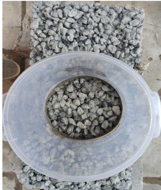
Fig. 5- Infiltration Rate Setup
