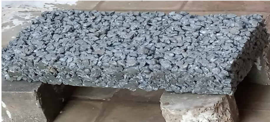
Fig. 6 – Pervious Concrete Slab
