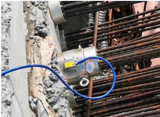
Fig. 5 - Field diagram of the pressure sensor
