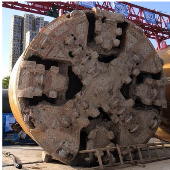
Fig. 3 – Pipe jacking machine
