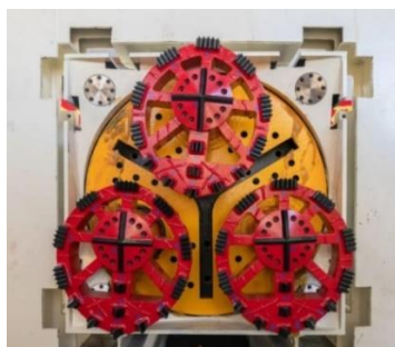
(a) Pipe jacking machine with three cutterheads (b) Pipe jacking machine with single cutterhead
