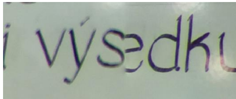
Fig. 6 – Bad stitching of images from camera rig
