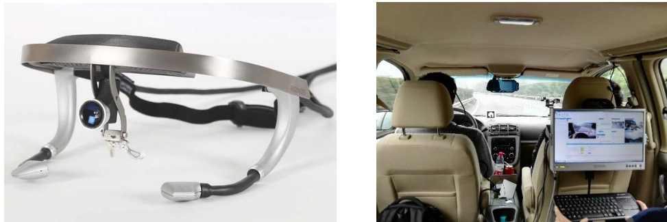
Fig. 1 - Eye movement instrument and on-board data processing equipment
