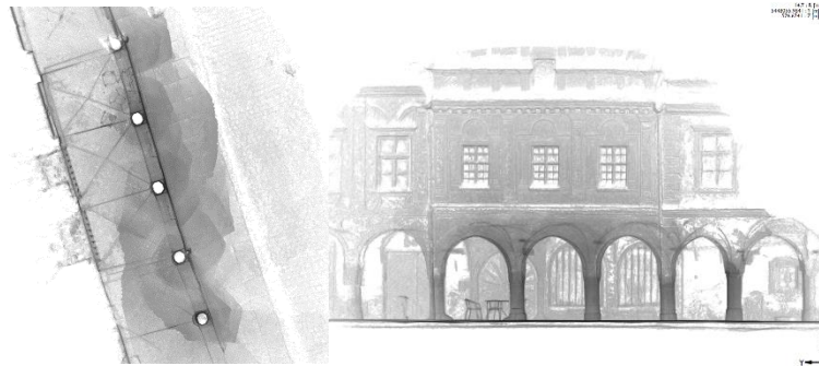
Fig.14 – View of the object and position of the moving device, plan view and side view created by projection of the point cloud from the ViDOC device.
