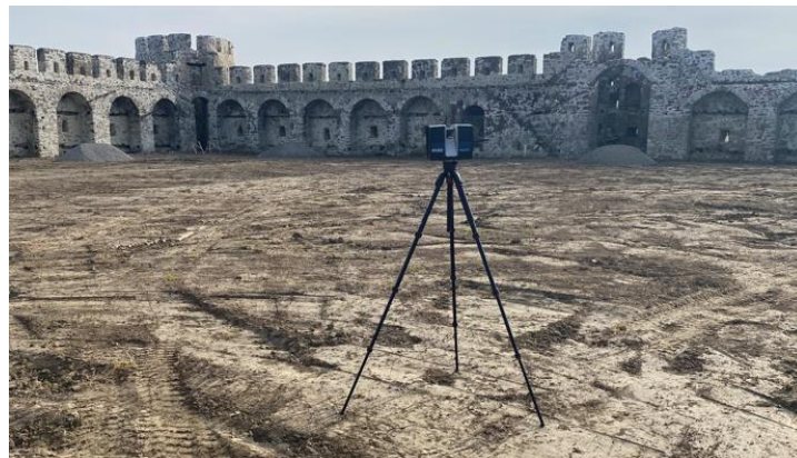
Fig. 7 – Laser Scanner Faro S70 during measurements inside the castle.
