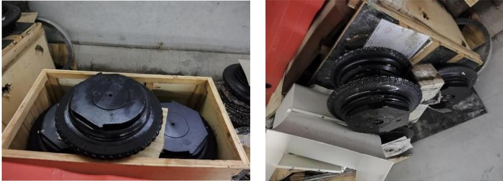
(a) Single-edge toothed roller cutter (b) Double-edge toothed roller cutter
