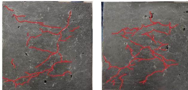
Fig. 2 - Polyurethane Cement Uniaxial Compression Failure Diagram
