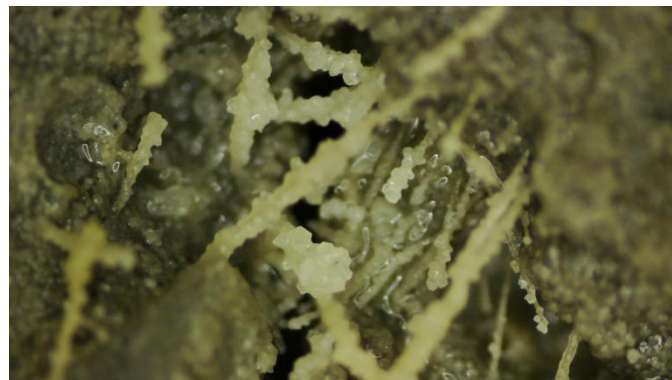
Fig. 15 - Calcium carbonate attaches to the surface of fibers
