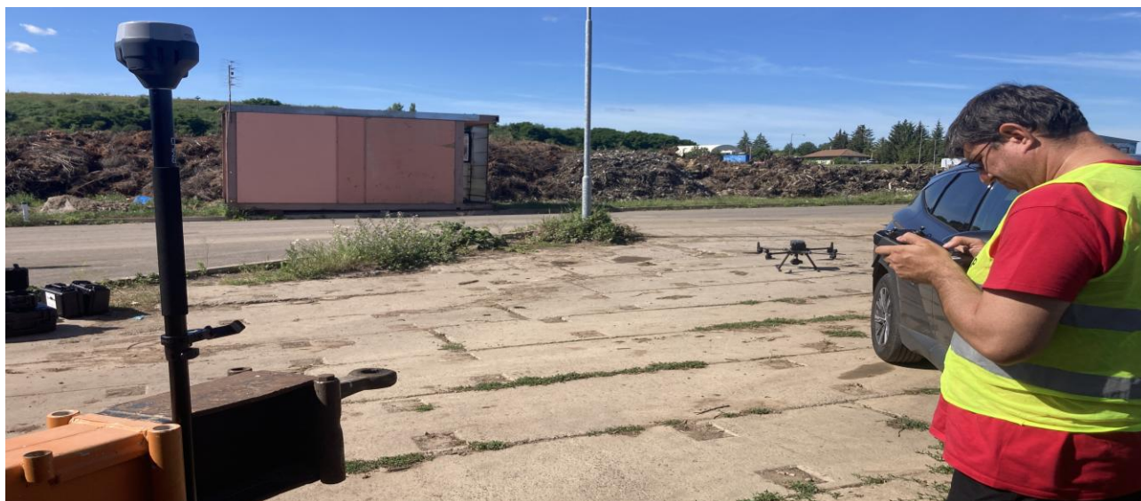
Fig.2 - Preparation by DJI M300, Emlid RS3 base station and 3gon Positioning worker, photo by O. Váňa
