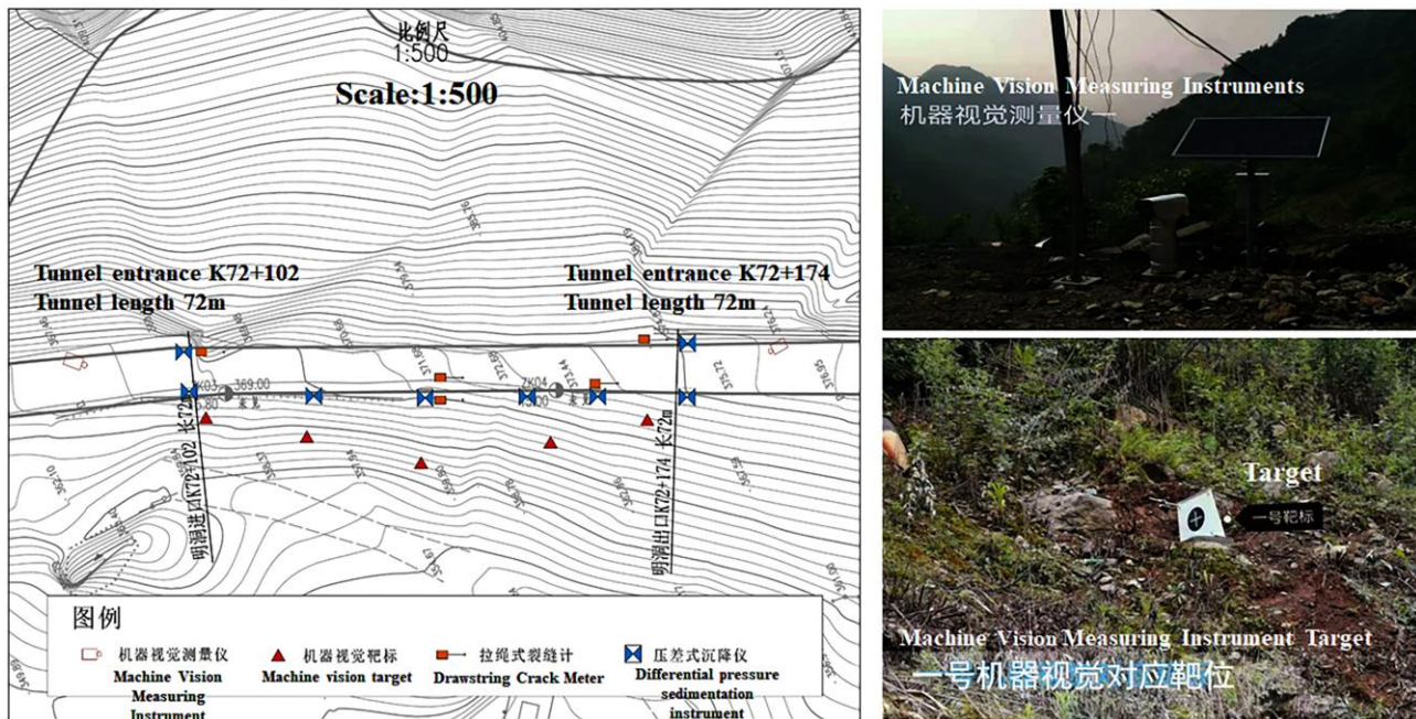
Fig. 9 - Layout of monitoring stations and monitoring sites
