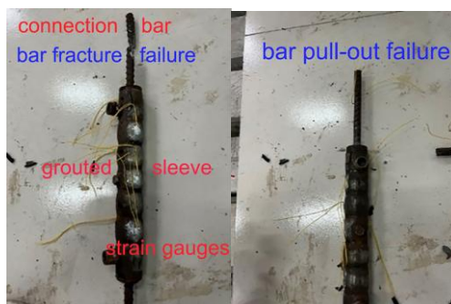
a) Bar fracture failure b) Bar pull-out failure
