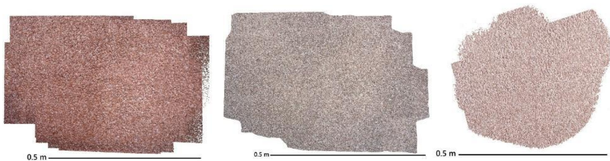
Fig. 18 – Dense cloud for Gravel 1 - software (from the left) Agisoft Metashape Professional, iTwin Capture Modeler a Pix4DMapper
