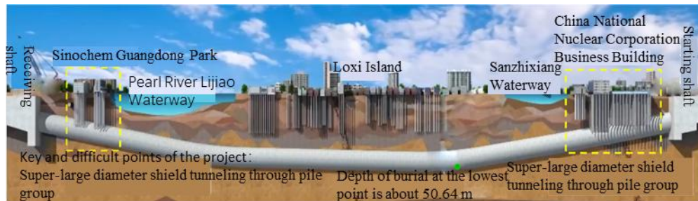
Fig. 1 - Engineering diagram of Haizhu Wan Tunnel shield section
