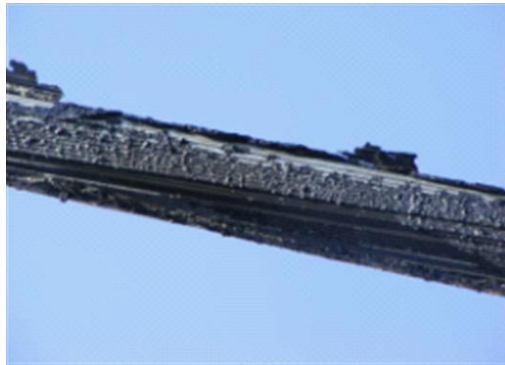
(a) - N12 cable fire damage diagram
