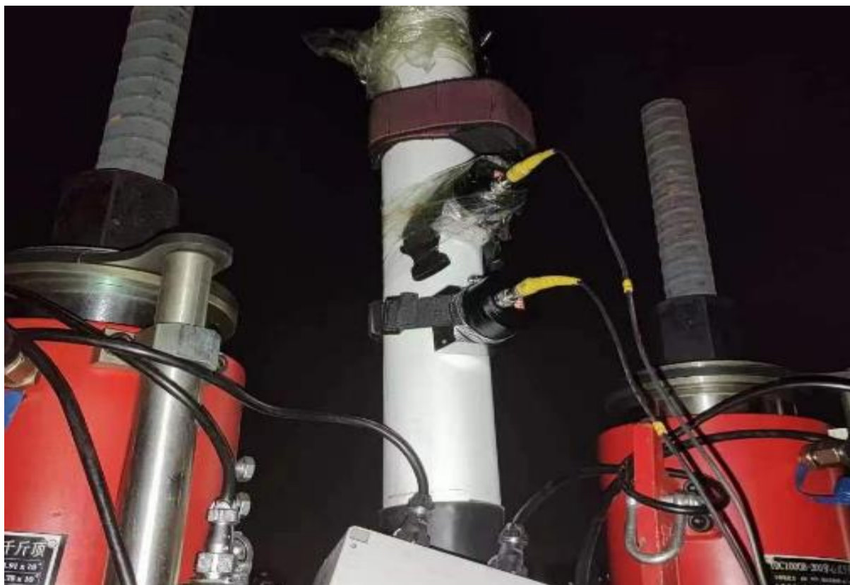
Fig. 6 – Cable force measurement
