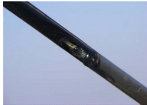
(b) - N13 cable fire damage diagram
