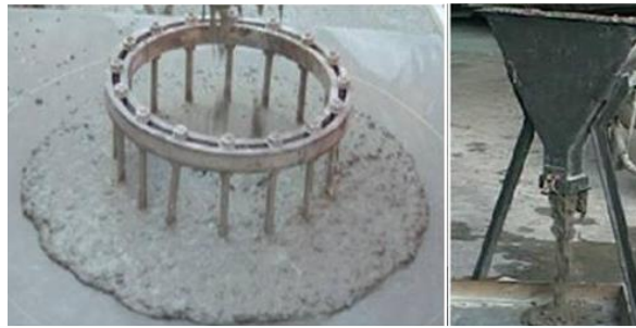
Fig. 3 - J-ring and V-funnel test [22]
