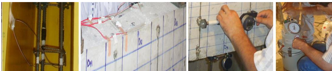
Fig. 8 - Application of measuring tapes, mechanical deformation and porosity measurement [11]
