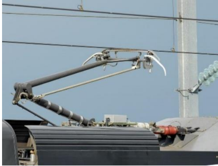
(a) overhead railway pantograph arm with tapered geometry
